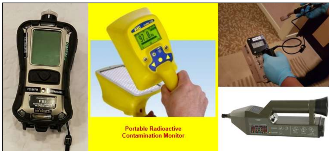
Figure 2.4 Examples of CBRNe Field Screening Tools (from left and clockwise - gas detector; portable radioactive contamination monitor; radiation survey meter; AP4C chemical detector)
